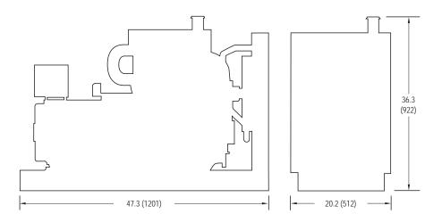
NL844W3 Overall Dimensions L x W x H: 47.3 x 20.2 x 36.3 inch (1201 x 512 x 922 mm) Base Lenght: 53.1 in (1349mm) Base Width: 21.21 in (540mm)
